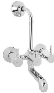
Cat No.: F60026 Wall Mixer with provision for Overhead Shower with 115 mm Long Bend Pipe & Wall Flange Brass Knob & Ceramic Disc : 3/4"
