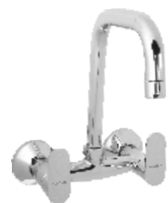
Cat No.: F61072 Sink Mixer with Extended Swivel Spout Brass Knob & Ceramic Disc : 3/4" (Wall Mounted) With Connecting Legs & Wall Flanges
