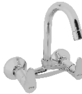
Cat No.: F62023 Sink Mixer with Normal Spout Brass Knob & Ceramic Disc : 3/4" (Wall Mounted) With Connecting Legs & Wall Flanges
