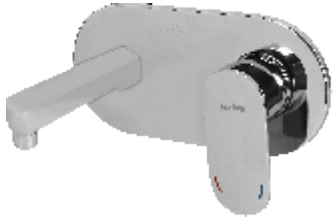
Cat No.: F61078 Exposed Part Kit of Single Lever Basin Mixer Wall Mounted consisting of Operator lever, Wall Flange, Nipple & Spout - Inspire (suitable for F85007)
