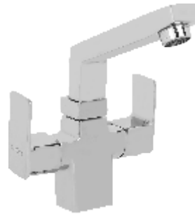
Cat No.: F62065 Center Hole Basin Mixer With Casted Spout Brass Knob & Ceramic Disc : 3/4" (W/o Popup Waste)
