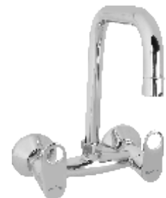
Cat No.: F60072 Sink Mixer with Extended Swivel Spout, Brass Knob & Ceramic Disc : 3/4" (Wall Mounted) With Connecting Legs & Wall Flanges
